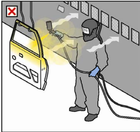
Figure 1 The operator is exposed to overspray because of poor positioning in relation to the airflow.
