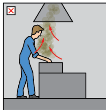
DIAGRAM 5 Poor design carries contaminants through the breathing zone.
