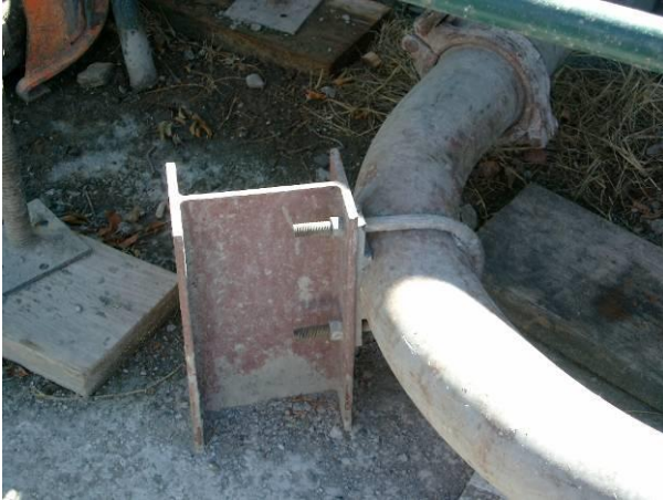
Figure 2. One method of anchoring pipe.
